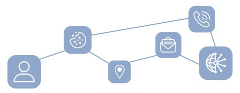
You can visualize a graph database as a series of hubs (also called nodes) and spokes (also called edges).
